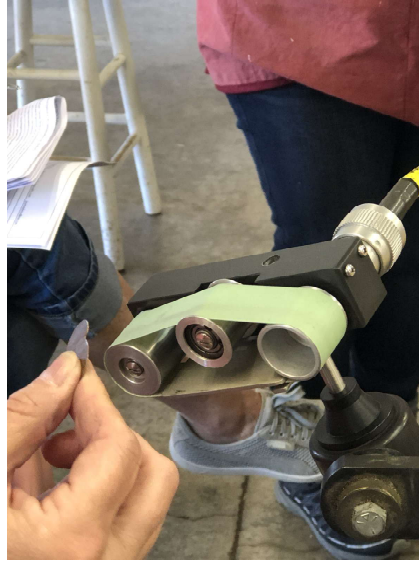
Jayne Redman demos cleaning up work on the Wolf Belt Sander add-on for flex shafts
